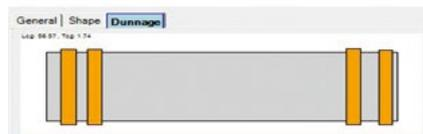
After loading a cargo unit, the dunnage creator allows planners to create a full range of related dunnage dividing the load into dunnage parts.
